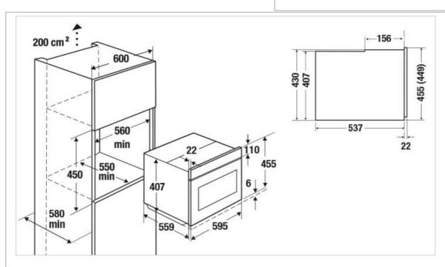
Minimum 200mm<sup>2</sup> at the back must be provided for ventilation.
